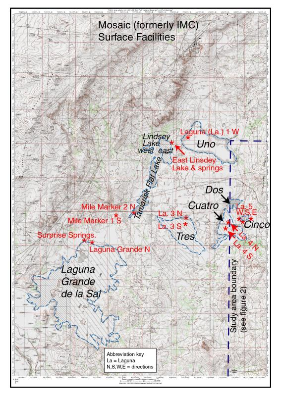
Figure 1. Brine ponds in southern Nash Draw. Red letters and asterisks identify general locations where historical specific gravity data have been collected since 1986. Major ponds are outlined with blue dashed lines.
